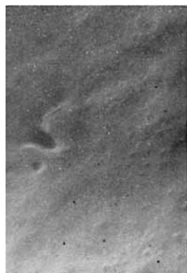
Fig. 4. As-molded Zytel 101; 38,300 \times .
