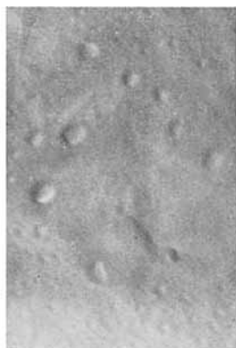
Fig. 5. Annealed Zytel 101 ( 150^{\circ}\text{C} .); 38,300 \times .
